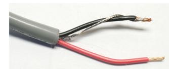
Black/Silver Wires Twisted & Insulation Removed
